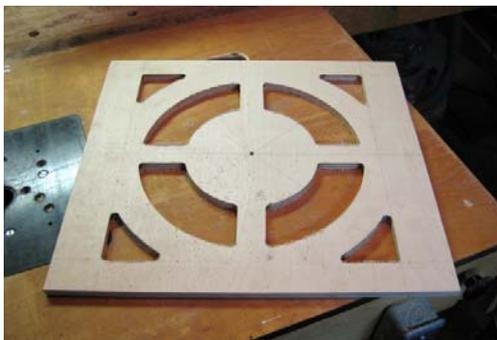
Figure 10 – The rocker box bottom piece.
