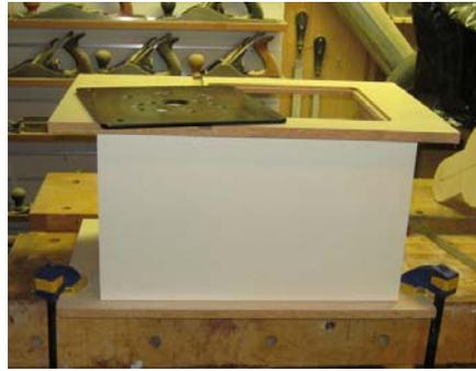
Figure 2 – A simple router table.
