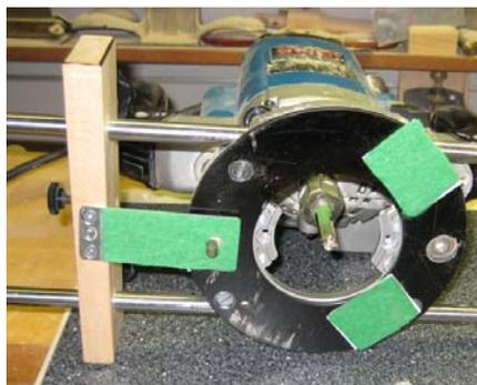
Figure 5 – A mod for cutting small circles.
