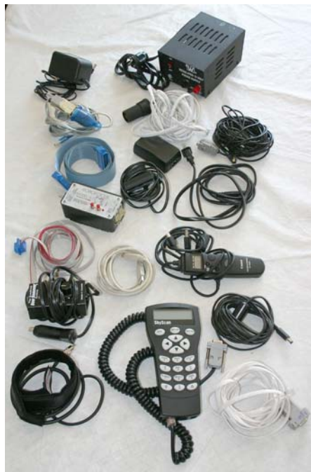
Figure 3. Just some of the power and data cables that need to be connected. Additional power supplies and cables are needed for the laptop, the autoguider and the autoguider control box.
