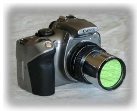
Figure 4. The Digital Rebel with T-ring, two-inch adapter and light pollution filter. This one's ready to slip into the focuser and go to work.
